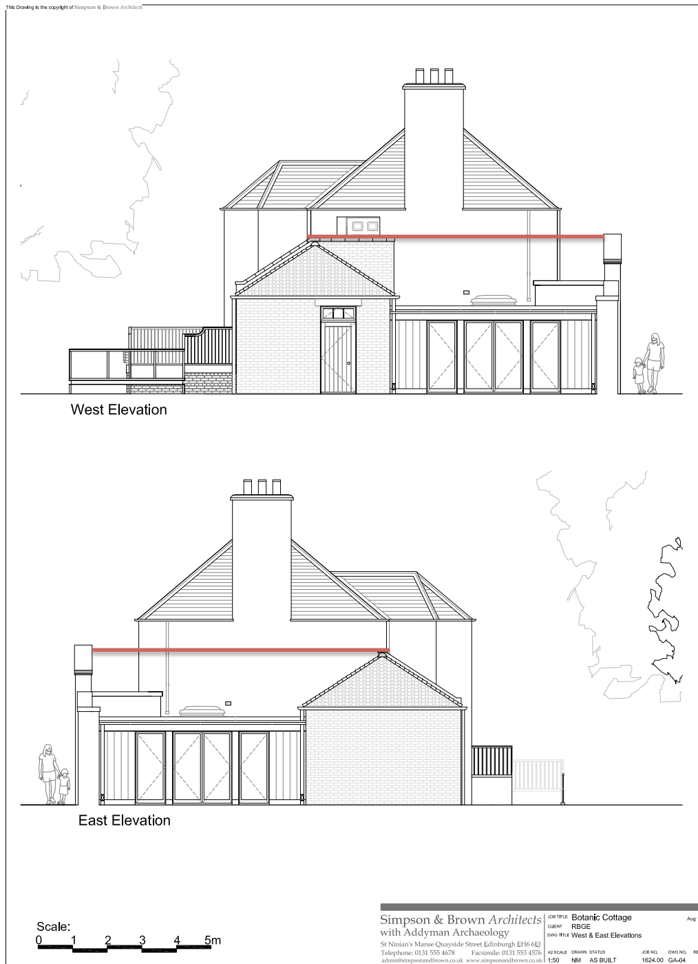
Fig 35: Plans of the Cottage by Simpson and Brown. The red lines show how the two additions were below the main façade. The West Elevation is the Garden Room while the East Elevation is the Potting Shed (After Simpson and Brown 2013, image courtesy of Neil McDonald).
